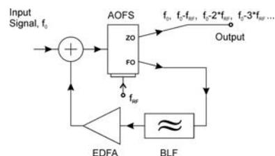
Fig. 1. The schematics of a multifrequency translator
