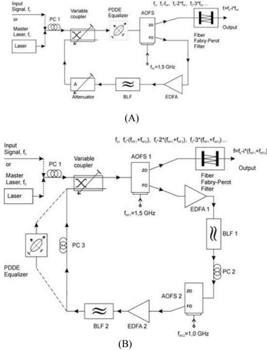
Fig. 2. Block diagrams of experimental setups: single shifter (A) and double shifter configuration (B)
