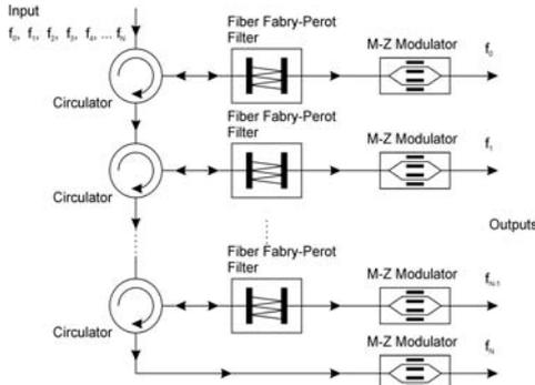
Fig. 5. Demultiplexer and modulation module, configuration with all fiber Fabry-Perot filter
