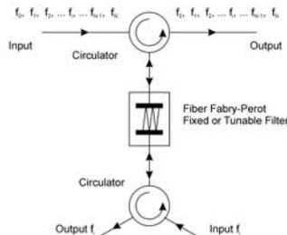
Fig. 6. Optical add/drop multiplexer, configuration with all fiber Fabry-Perot filter
