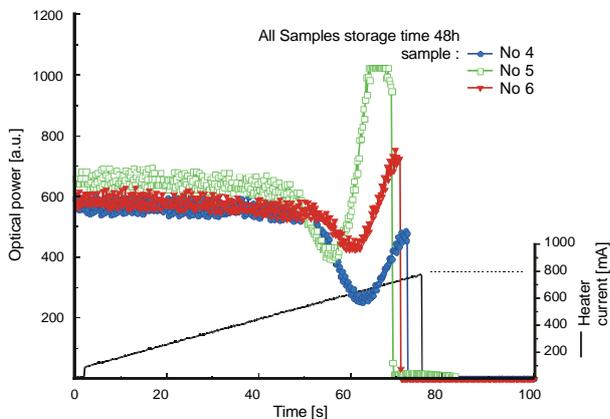
Fig. 3. Optical signal received during local heating from nephelometric arm for milk stored for 48 hrs, at 21° C.
