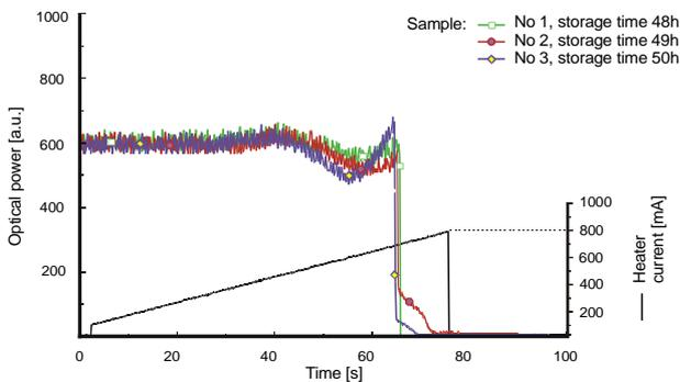
Fig. 2. Optical signal received during local heating from nephelometric arm for milk stored for 48, 49, 50 hrs at 10° C.
