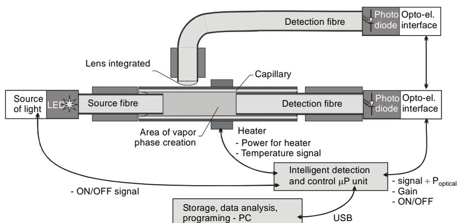
Fig. 1. Sensor configuration for the microlitre sample analysis of milk.
