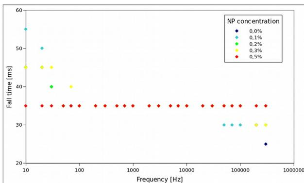
Fig. 3. PLCF fall times induced by external electric field for wide frequencies range
