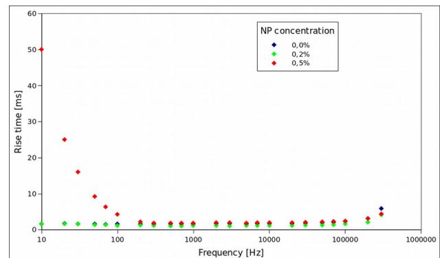
Fig. 4. PLCF rise times induced by external electric field for wide frequencies range for concentrations 0.5% wt. to 0.2% wt. and 0% wt.
