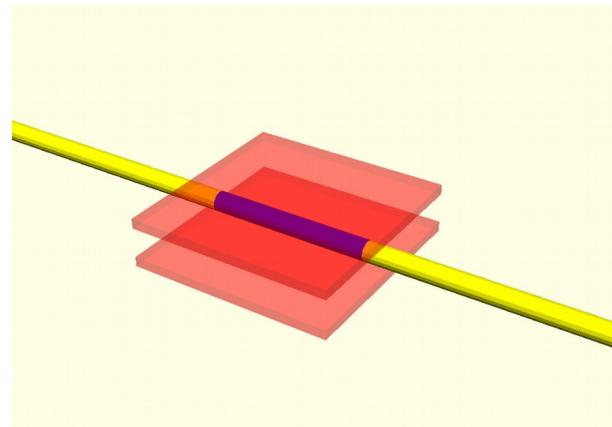
*Fig. 1. Setup of PLCF (blue section of yellow optical fiber) with NP-doped LC response for electric field with various modulation frequencies placed between two plates (red)*
