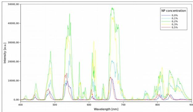
Fig. 2. Transsmision spectra for PCF infiltrated with Au NP doped LC
