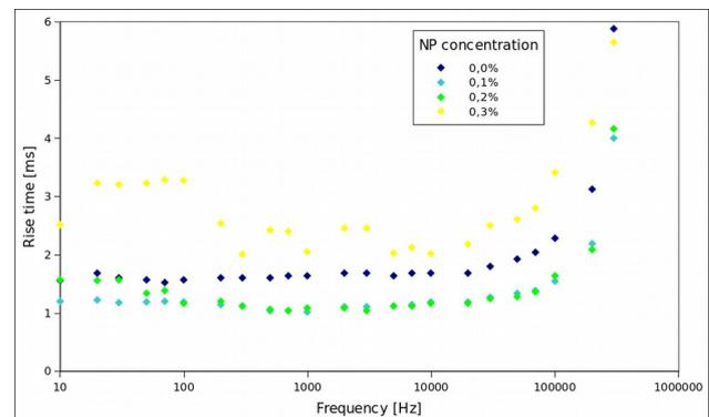
Fig. 5. PLCF rise times induced by external electric field for wide frequencies range for concentrations 0% wt. - 0.3% wt..
