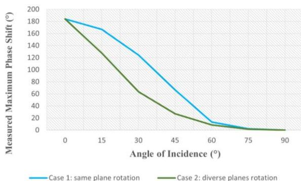
Fig. 6. Experimentally measured differential phase shift at 10 GHz versus incident angles. Measurement results based on setup maintaining laser driving current of 3 A and delay line device position fixed.
