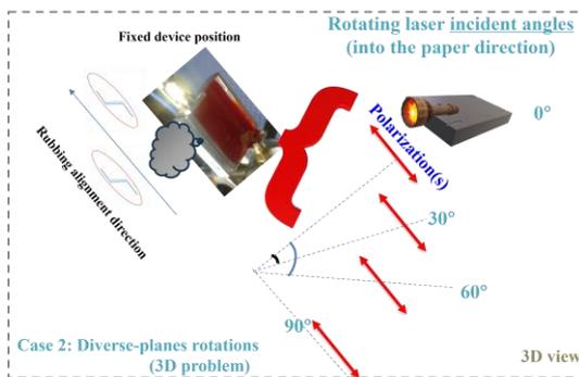
Fig. 5. Core experimental approach in incident angle study (2D view represents resulting laser polarizations rotated in diverse planes relative to fixed rubbing alignment direction). Measurement results based on setup maintaining laser driving current of 3 A.
