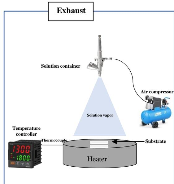
Fig.1. schematic diagram of spray pyrolysis technique.
