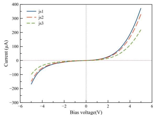
Fig. 4. I-V characteristics in the dark for p-Si/n-CdSe at different thicknesses of the CdSe layer.
