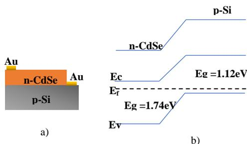
Fig. 3. (a) The schematic structure of the n-CdSe/p-Si heterojunction and (b) the band gap structure of the n-CdSe/p-Si heterojunction.
