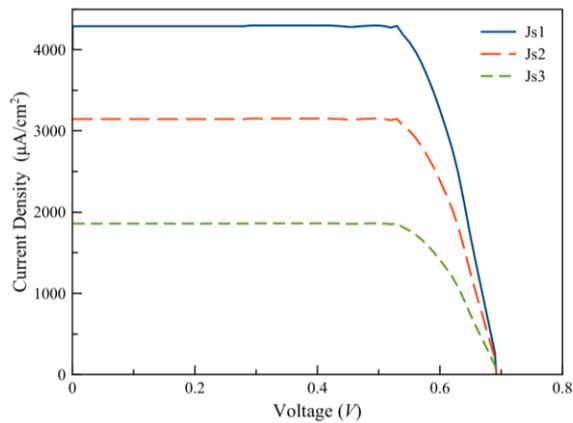
Fig. 5. I-V curve of the p-Si/ n-CdSe heterostructure cell under illumination at different thicknesses of the CdSe layer.
