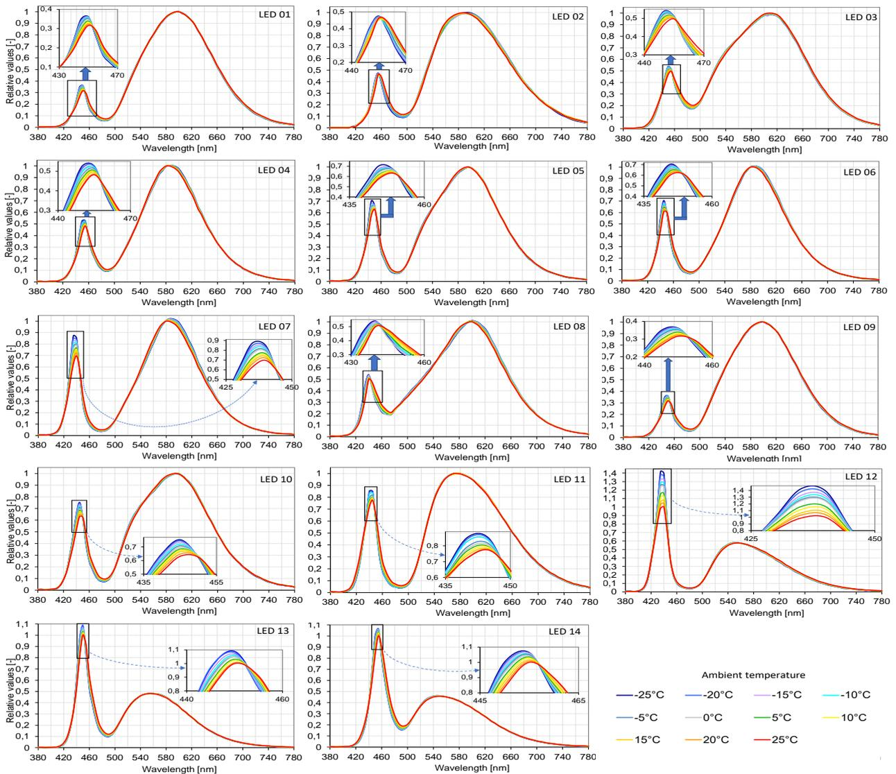
Fig. 1. Relative spectral characteristics of 14 LED sources for various ambient temperatures.
