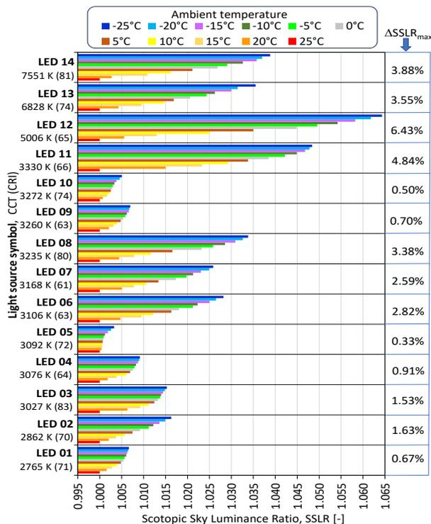
Fig. 2. Graphic visualization of calculated SSLR indices for 14 LED lamps operating at various ambient temperatures.
