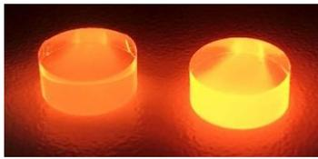
Fig. 1. Fabricated nanocomposite probes sample 1 (left) and sample 3 (right) under exposition to UV LED (365 nm).
