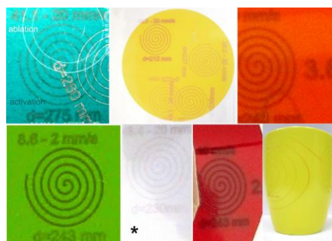
Fig. 8. Examples of activation for selected glaze colours of ceramic products. The asterisk indicates the white glaze used in typical tableware.
